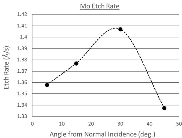
Fig. 1. Etch rate of Mo films versus stage angle with  $V_b = 300$  V,  $I_b = 115$  mA, and  $V_a = 36$  V.
