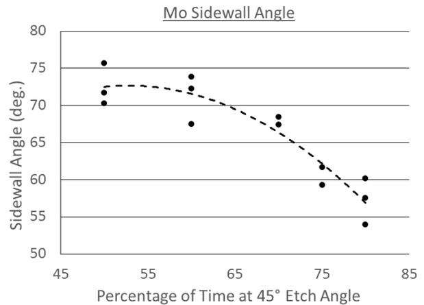
Fig. 2. Mo IBE sidewall angle as a function of etching time spent at an initial angle of  $45^\circ$ . The remainder of the etch is carried at  $5^\circ$ .
