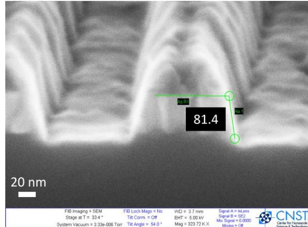
Fig. 5. Cr sidewall angle of 81.4° after etching 30% time at 45°. A thin layer of photoresist remains above Cr material.
