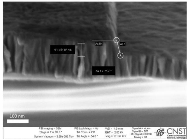
Fig. 3. Mo sidewall angle after etching 50% at  $45^\circ$  and 50% at  $5^\circ$ .
