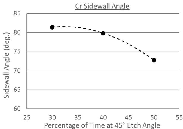
Fig. 4. Cr IBE sidewall angle as a function of etching time spent at an initial angle of 45°.
