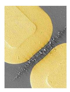
Image showing a scanning electron microscope image of damaged vanadium dioxide in the gap of a terahertz metamaterial made of gold. The damage results when strong field enhancement of incident terahertz radiation in the gaps leads to a rapid increase in the energy density following the field-driven insulator-to-metal transition. Image Credit: Mengkun Liu / Mario D'Amato
